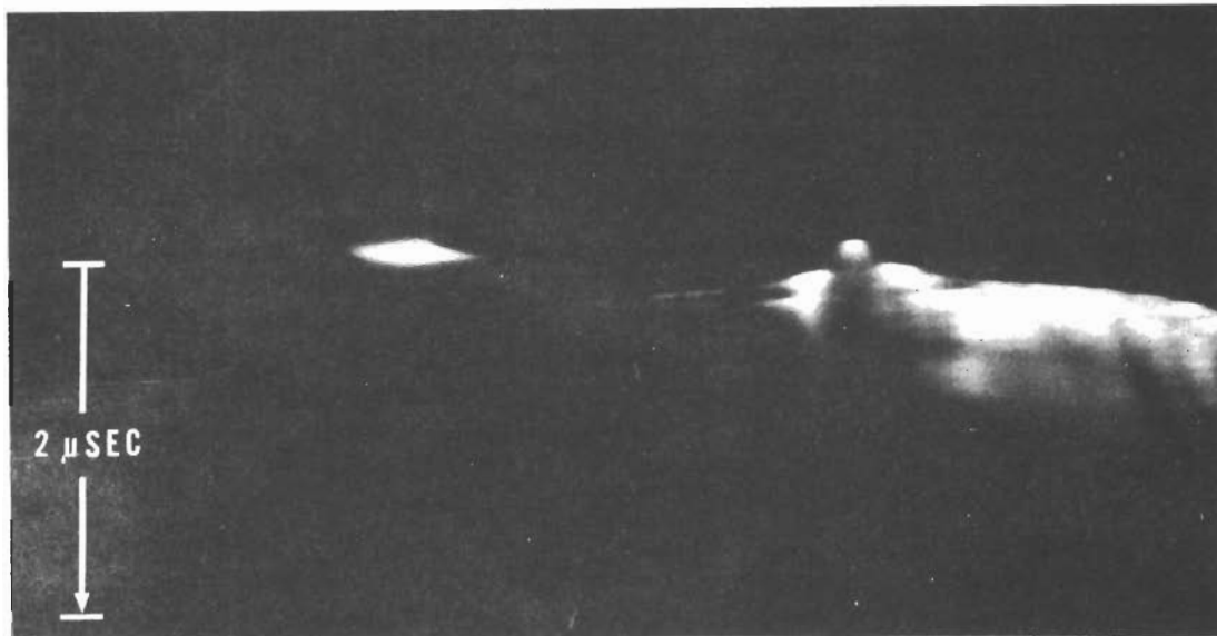
Fig. 17 RMC photograph viewing plane shock traveling from left to right through the assembly shown above. The space between the glass plate and the prism was evacuated. The burst of light seen on the prism face is opposite the triangular groove in the glass plate.
